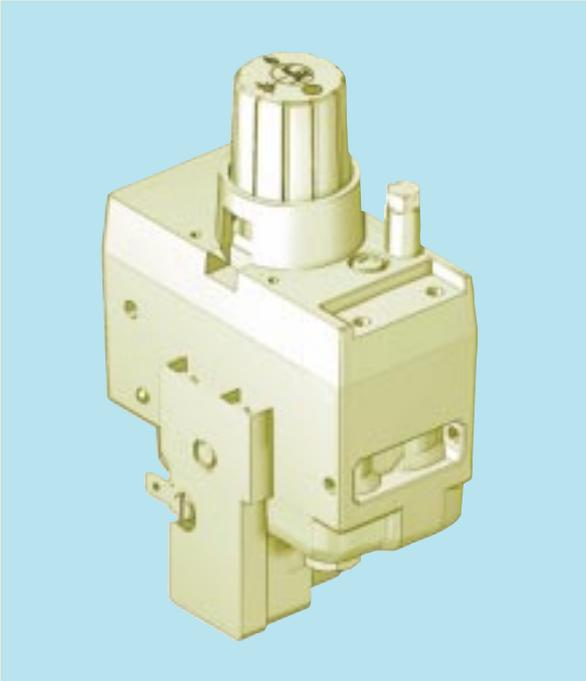
**Multifunctional single-knob control (off, pilot, on) with thermoelectric safety device and near silent ON-OFF solenoid valve. Facility to mount a piezo-electric igniter.**
